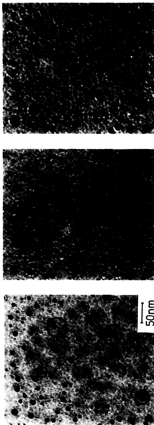
FIG. 3. Micrographs of Ni/Al 2 O 3 heated in H 2 at 600°C for 1 h and then in O 2 (a) at 100°C for 12 min, (b) at 150°C for 11 min, and (c) at 200°C for 10 min. The circles indicate the same region of the specimen.
